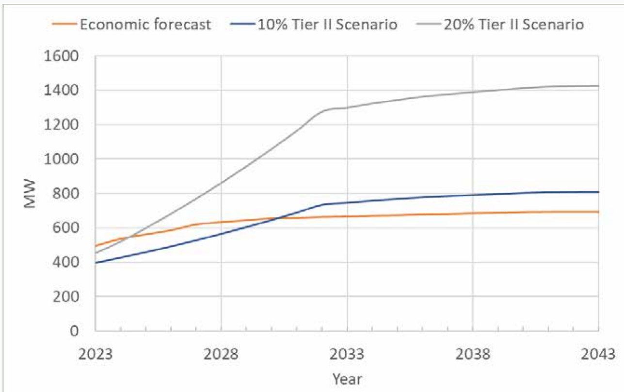
FIGURE 9 - SOLAR PV IMPACT ON VERMONT NET LOADS
