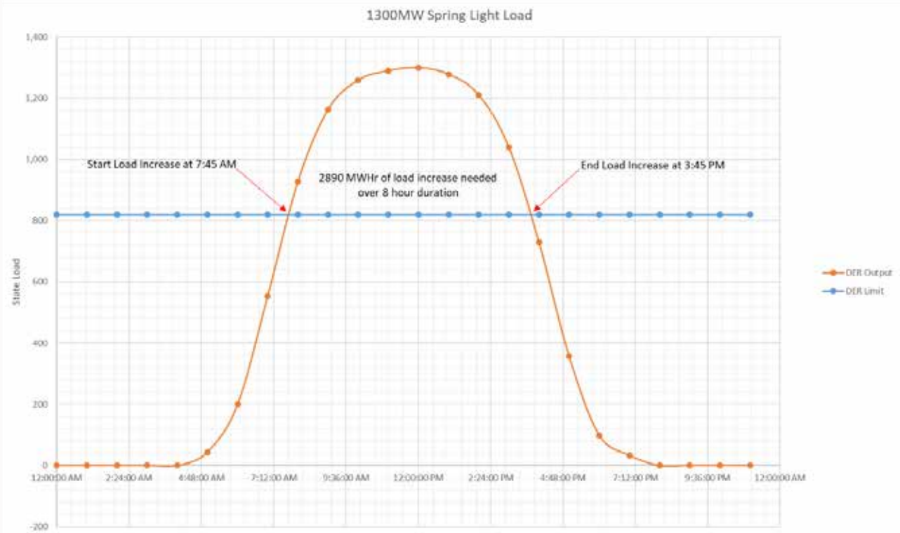
FIGURE 21 - ENERGY ESTIMATE OF AGGREGATE STORAGE OR LOAD CONTROL FOR DG IMPACT MITIGATION
