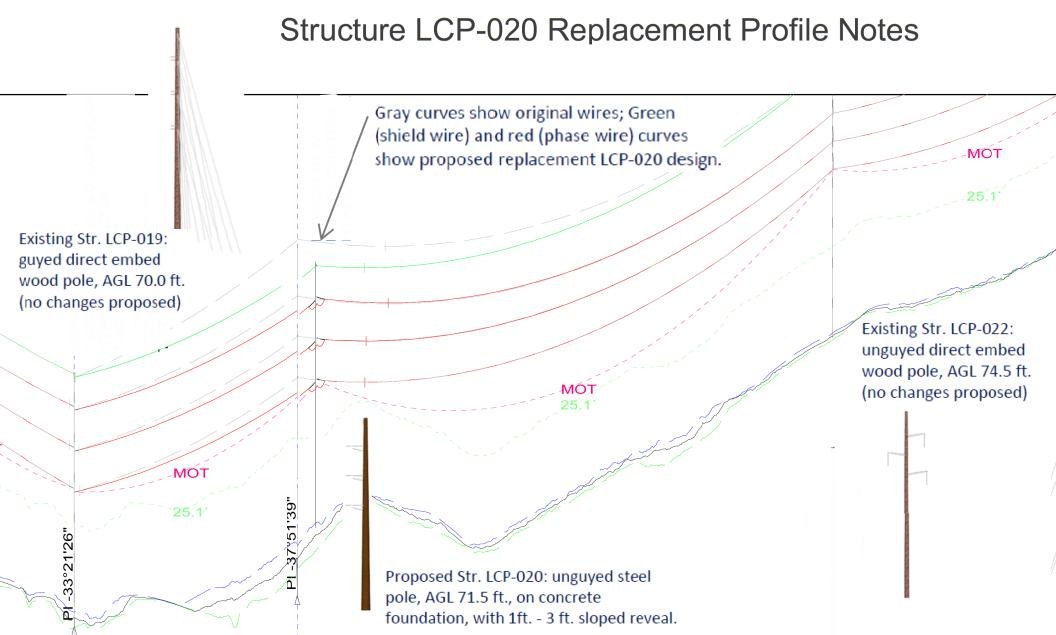
MOT = Maximum Operating Temperature; curves shown for approx. 40 d. F; 25.1' = Ground Clearance Min. Design Basis; PI = Point of Inflection (Line Angle); AGL = Above Grade Length; Blue/Black/Green Gradelines = 15' Left/Centerline/15' Right profiles.
